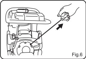
4 After the engine has started, open the choke lever gradually until it is wide open. Pay attention to the sound of the engine to guide you in the amount to open the choke. After the engine has started, be sure to warm up the engine at low speed for 3 to 5 minutes. During this time, check the machine for leaking fuel, abnormal sounds, or abnormal exhaust color or odor.
