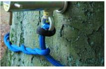
(6) Secure the device using a sufficiently rated Dead-Eye or Whoopie Sling. This is to be connected directly to the base anchor point as shown in the diagram. If you are using a Dead-Eye tie off using a suitable hitch.
