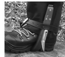
(5) Fasten the ankle straps ensuring the strap is not twisted and passes around the climber shank and above the top of the gaff
