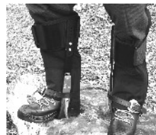
(8) Test the climbers are securely fastened and positioned correctly before commencing to climb. Readjust the climbers if required
