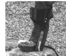
(3) Stand firmly in the climbers ensuring you have positioned them on the correct leg
