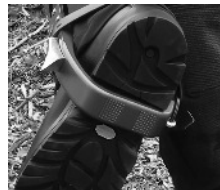
(4) The climber should fit securely against the heel of your boots
